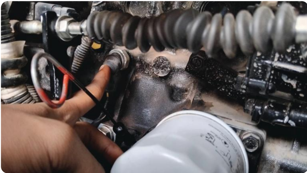
Gambar 1.21 Posisi Oil Pressure Pickup Plug
