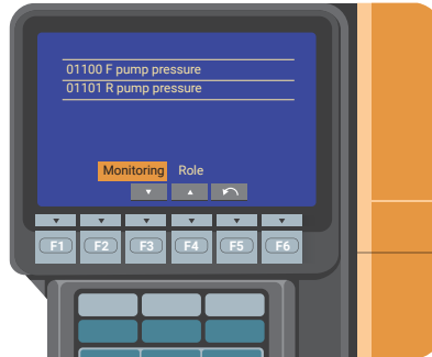
Gambar 2.27 Menu Machine Monitor Pengukuran Tekanan Hydraulic
